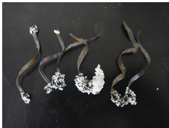
Figure 4. The appearances of the stainless-steel strips after microwave discharge.
